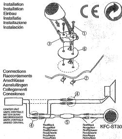
When making connection by cutting the speaker cord which was originally installed in the vehicle, use accessory (4).
